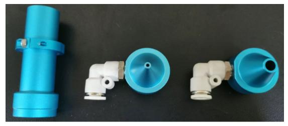
A nozzle has a very narrow outlet (approx. 2mm), which provides high air flow to blow directly on the cutting gap. This nozzle is excellently suited for cutting wood, as this prevents soot formation in the cutting gap.
