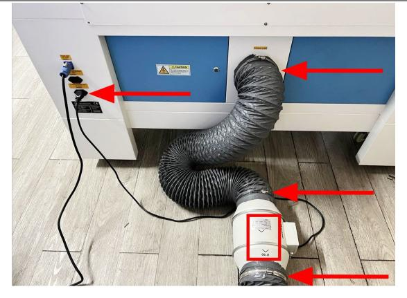
Also you can refer to the video on how to set up your Nova laser machine in our website <u>http://www.thunderlaser.com/how-to-use-your-laser-machine/how-to-setup-your-nova-laser-cutter.html</u> The input voltage must correspond (AC 230V 50/60 Hz or AC 115V 50/60 Hz) – see information label beside the connection socket.
