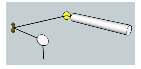
After being used for a long time, the beam path might be deflective. This will reduce the efficient of the laser beam or even cause no laser beam. At this moment, you will need to re-adjust the beam path again.
