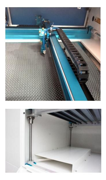
It is suggested to add lubricant oil (or Rust Preventative Grease) to the rails/screws at least every two weeks.
