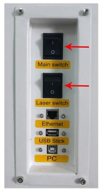
If all covers are closed, immediately after being switched on, the device starts the referencing process. When the referencing process is completed correctly, an acoustic signal sounds and the device is ready for operation. The operation panel will display the home screen when the laser is completed resets.
