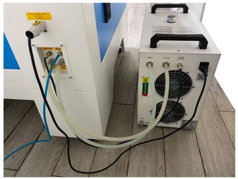
6 Add pure (distilled) water into the chiller until the water level in the green area showing on the gauge. Run chiller for a period of time, the water will fill into the laser tube on the machine, please re-add water to keep the water level in the green area.
