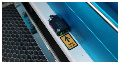
Move the table down till there's enough space, then place the material between the auto focus sensors. Make sure you always insert as far as the laser head stops by the ring. After that, go into Menu button>>Select Auto Focus.
