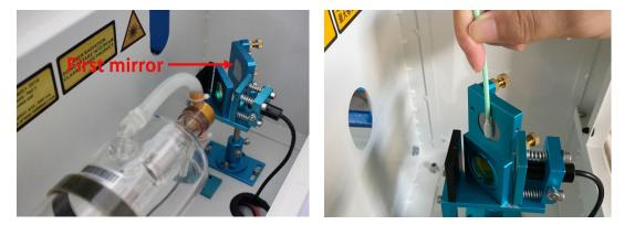
The 1<sup>st</sup> mirror is installed in the rear box of the laser tube, open it then view the right side.
