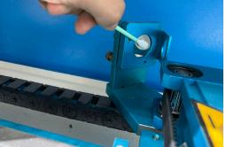
The 2<sup>nd</sup> mirror is installed on the left side of X rail.
