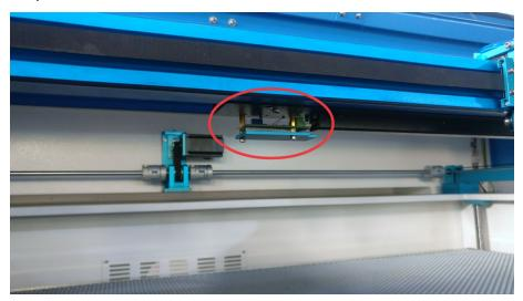
The warning sound comes from signal lamp (roughly 80dBA within 1m, 75dBA within 5m and 65dBA within 10m, the sound gets weaker as it travels).
