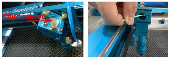
The 3<sup>rd</sup> mirror is installed on the top of the laser head.
