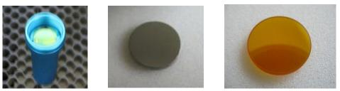
It is suggested to clean the mirrors/lens before work every day in order to run the machine at max efficiency. Please turn off the power of laser machine before cleaning the optical parts.
