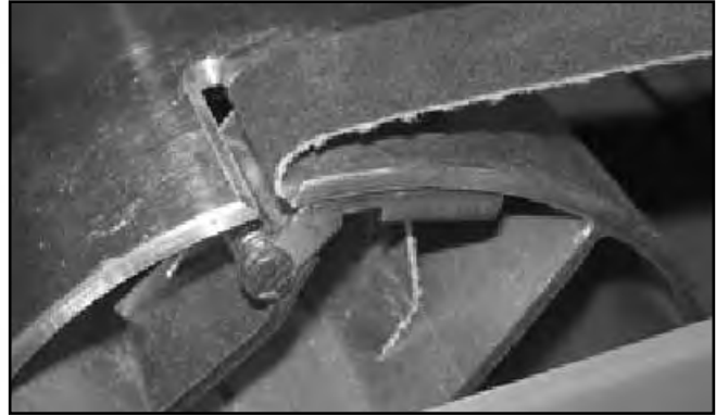
2. Insert the left tab of the sanding belt in the slot, pushing all the way in (as far as possible), then release the clamp to lock the tab in place.
