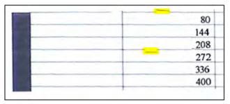
On the left of each Printhead Nozzle test, there is a series of horizontal straight lines. If one or more nozzles are misdirected there will be unequal spaces between the corresponding lines.
