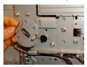
28. Disconnect the Pinchwheel Lifter Sensor, and unroute the cable.
