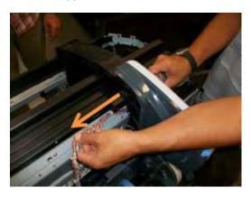
16. Detach the cable from the cable tie.
