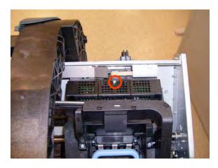
6. Remove the small cover of the Carriage PCA.
