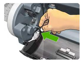
Insert the Lower Roll Cover left-side hinge into the Lower Left Roll Support pin. 6.
