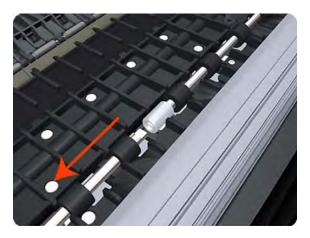
**10.** Carefully lift the left Print Zone Overdrive out of the printer.
