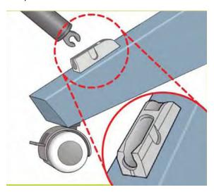
5. Attach the basket's front tubes to the two short tubes on each foot.
