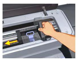
9. Clean the part of the encoder strip inside the Service Station by repeating steps 2 to 6.
