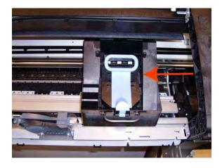
12. Remove the cover on each side of the Carriage PCA using a screwdriver to unclip it.
