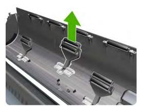
5. Locate the new pinch arm assembly and screws.
