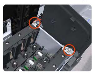
6. Remove the two Left Ink Supply Station bonding cables.
