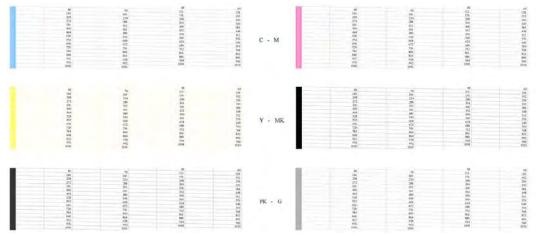
If any nozzles are not printing correctly they will be shown on the right of each Printhead Nozzle test. There is a series of numbered stepped diagonal lines. If one or more of the nozzles are clogged, malfunctioning or mis-positioned, you will see that the stepped lines are broken or misdirected in one or more places.
