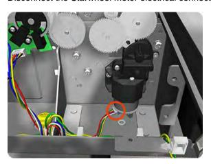
7. Carefully pull the two gear wheels off their shafts to gain access to the Starwheel Motor attachment screws.
