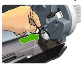
Screw the Lower Roll Cover to the Lower Right Roll Support. **7**.
