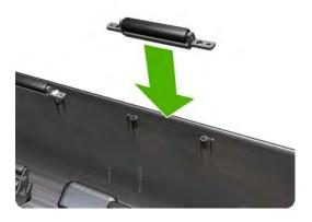
6. Screw the freewheel assembly to the roll cover.
