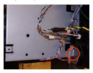
5. Remove the grounding cable attachment T-10 screw from the metal sideplate.
