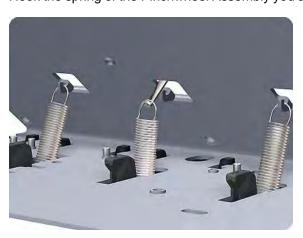
4. Attach the spring to its attachment point on the hanger and remove the Pinchwheel Insertion Tool.
