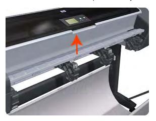
6. Slide the Media Output Assembly forwards out of the printer.
