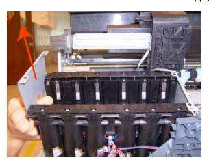
21. Remove two T-10 screws that secure the Right Side Plate of the Left Ink Supply Station.
