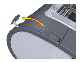
7. Use the Pinchwheel Insertion Tool to remove the spring from the attachment on the printer.
