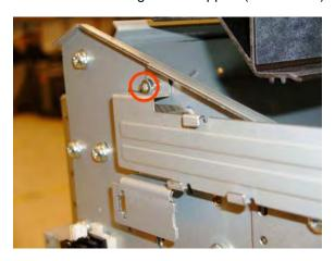
**30.** Remove the Trailing Cable support.
