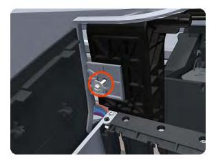
**11.** Carefully pull the attachment clip forward until you can lift the bottom left corner of the Top Cover approximately 10 mm.
