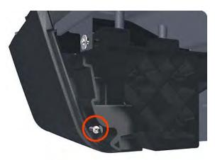
13. Remove one T-15 screw that secures the Left Cover (top front, accessible Ink Cartridge Door).
