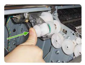
6. While maintaining pressure on the Media Advance Drive Adjustment Tool, fully tighten the three T-15 attachment screws in the order shown.
