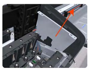
8. Remove the T-20 screw that secures the Left Ink Supply Station to the printer.
