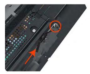
12. Rotate the Carriage Rear Bushing vertically and remove it from the Carriage Assembly.
