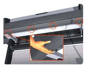
3. Carefully pull the bottom of the Front Cover forwards until you can release it from its attachments.
