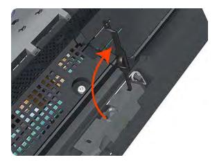
NOTE: When you reinstall the Carriage Rear Bushing, use the Oil and Oil Dispenser from the Lubrication Kit to add 2 or 3 drops of oil to the small depression in it.
