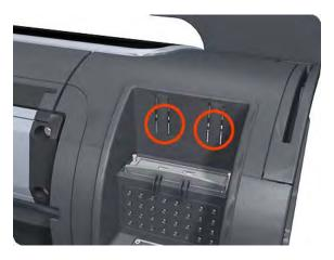
8. Lift the Formatter Housing out of the printer.
