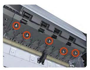
7. Lower the left end and remove the Left Roll Guide from the printer.
