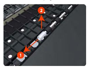
**12.** Use a flat-bladed screwdriver to unclip the left Print Zone Overdrive retaining clip and rotate the clip vertically.
