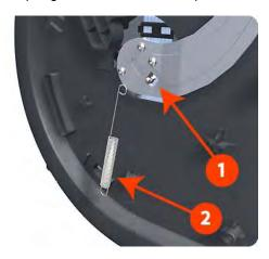
Remove three T-15 screws that secure the Media Lever.
