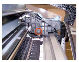
21. Remove the Line Sensor from Carriage Assembly.
