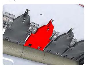
14. Collapse the Pinchwheel Alignment Tool to remove it.
