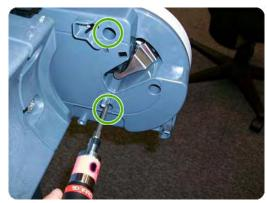
Unplug the Lower Left Roll Support, taking care not to damage the cables. 6.
