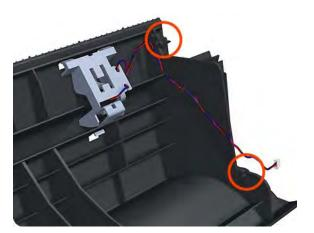
5. Unroute (unwind) the Out Of Paper Sensor electrical cables from the Out Of Paper Sensor cover.
