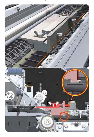
10. Loosen the wing nuts on the Pinchwheel Alignment Tool.
