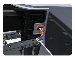
9. Carefully pull the attachment clip forward until you can lift the bottom left corner of the Top Cover approximately 10 mm.
