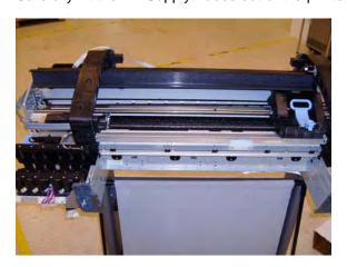
**25.** Carefully remove the Ink Supply Tubes from the assembly.
