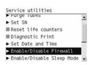
2. The Front Panel tells you whether the firewall is currently enabled or disabled, and allows you to change its status by pressing the **Up** and **Down** keys and then the **OK** key.
