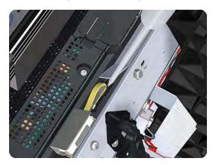
NOTE: When you reinstall the Carriage Rail Oiler, use the Oil and Oil Dispenser from the Lubrication Kit to add 2 or 3 drops of oil to the foam of the Carriage Rail Oiler and in the small depression of the Carriage Rear Bushing.
