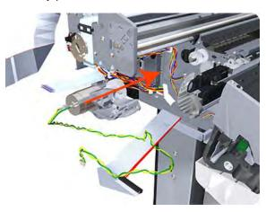
2. Insert the three T-15 attachment screws, but do **not** fully tighten them.
