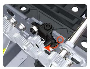
9. Tilt the Left Starwheel Lifter sufficiently to disengage the left attachment lug.
