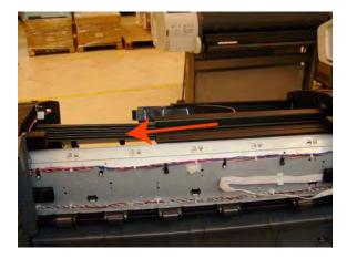
9. Remove the Ink Supply Tubes Support Rail from the printer.
