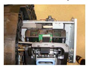
7. Disconnect the ribbon Trailing Cable from the Carriage PCA.
