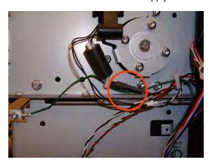
12. Remove three T-20 screws that secure the Scan-Axis Motor to the printer.
