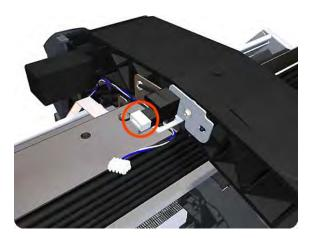
8. Remove one T-15 screw that secures the Window Position Sensor to the printer.
