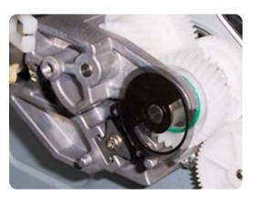
3. Press the encoder using the Media Advance Drive Adjustment Tool (reversed) so that it sticks to the roller.
