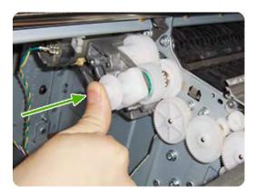
5. While maintaining pressure on the Media Advance Drive Adjustment Tool, fully tighten the three T-15 attachment screws in the order shown.
