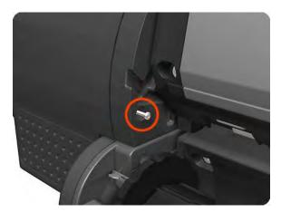
6. Remove one T-15 screw that secures the Right Cover to the printer (at the rear of the printer).
