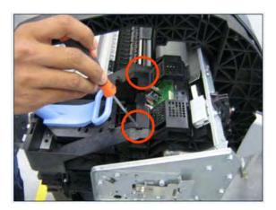
13. Disconnect the 6 ribbon cables of the Carriage Cover from the Carriage Assembly PCB.
