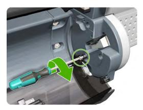
Close the Lower Roll Cover until the other end of the Bi-stable Screw is in front of the hole on the Lower Left Roll Support (if necessary, hold the Roll Cover for a moment with your head).
