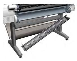
12. Hold the roll cover with one hand while unscrewing the other bi-stable spring from the printer.
