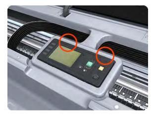
4. Rotate the front panel vertically.
