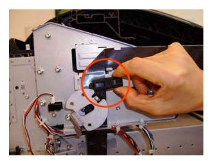
12. Remove 3 Cable Clamps, then unroute the Trailing Cables.
