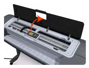
3. Squeeze the top edge of the front panel strongly enough to release the attachment clips, and begin rotating the Front Panel vertically in the next step.
