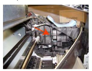
20. Remove one T-10 screw that secures the Line Sensor to the Carriage Assembly.
