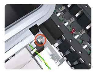
9. Remove the two T-20 screws that secure the Left Ink Supply Station to the printer.
