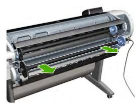
3. Remove the screw connecting the roll cover to the printer on the left.
