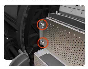
9. Remove one T-20 screw that secures the Electronics Module to the printer.
