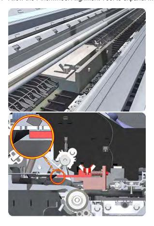
**12.** When the Pinchwheel Alignment Tool is fully expanded, the Pinchwheel Assembly is properly aligned.
