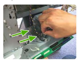
11. Remove the EE box from the printer.
