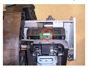
**18.** Open the latch, and remove the four T-15 screws that secure the Ink Supply Tubes to the Carriage Assembly.
