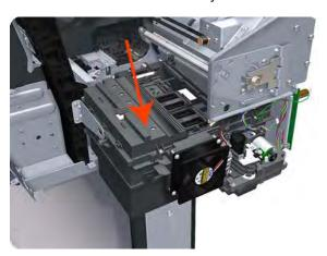
13. Carefully slide the Service Station from the printer.
