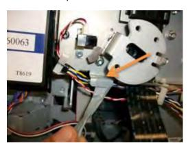
9. Remove the RFID tag support.
