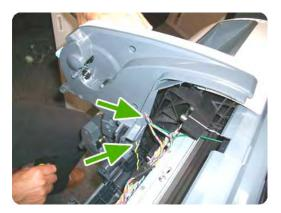
6. Disconnect the cable connector as shown.
