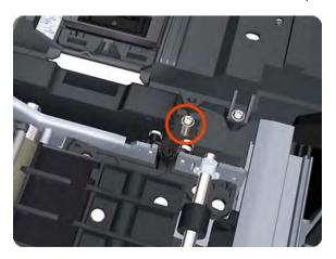
7. Rotate the Drop Detector vertically to gain access to the two screws that secure the Right Starwheel Lifter.
