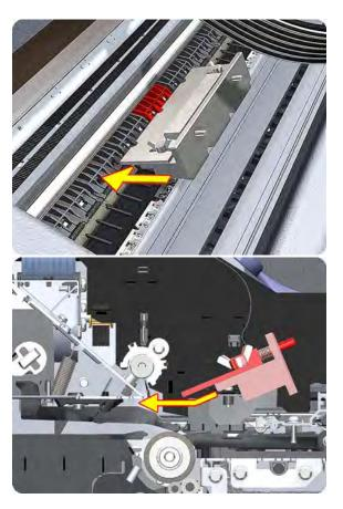
9. Set the Pinchwheel Alignment Tool on the print platen. The tool should fit as shown below.
