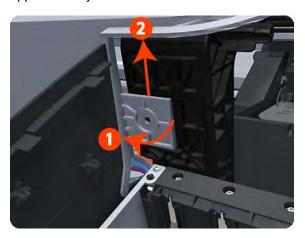
12. Lift the Top Cover of the printer sufficiently to gain access to the Front Panel ribbon cable.
