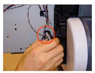
**8.** Push the Carriage Assembly into the print path.
