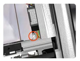
10. Carefully lift the Electronics Module out of the printer.
