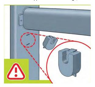
**4.** Fit the two short tubes to the printer's feet, one on the front of each foot. Each tube should click into place.
