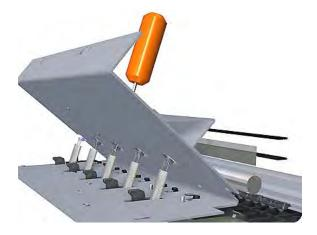
**5.** Attach the new Pinchwheel Assembly with the two T-15 screws that secure to the printer but do fully **not** tighten the screws.
