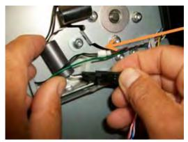
**24.** Pull the lower cable branch back under the right arc.
