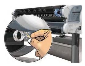
14. Free the other end of the right metal link of the right Bi-stable Spring (if necessary, play slightly with the Lower Roll Cover).
