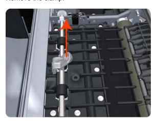
**6.** Repeat the three preceding steps to remove the remaining five attachment clamps.
