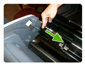
5. Remove the Roll Cover hinge from the Roll Right Support Pin.
