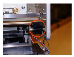
7. Secure the right bumper to the printer with a T-15 screw.
