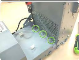
3. Remove the PSU module from the EE box base.
