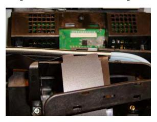
12. Slide the Trailing Cables out of the attachment clips of the Carriage Assembly.
