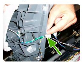
6. Disconnect the cable connector as shown.
