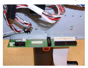
5. Remove two T-20 screws that secure the Electronics Module to the printer.
