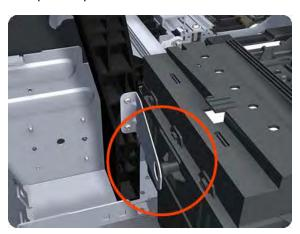
**12.** Lower the Service Station until you can slide it carefully from the printer.
