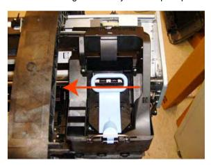
9. Unclip the Encoder Strip tensioner from the right hand end and pull the encoder strip straight out.
