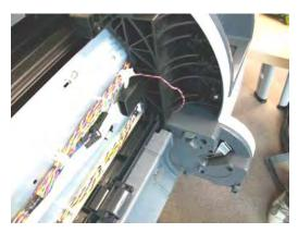
**7**. Disconnect the cable connector as shown.
