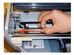
6. Unclip the Encoder Strip from its attachment lugs.
