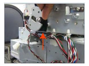
17. Unclip and remove the four cable clamps from the Trailing Cables.
