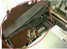
5. Secure the left bumper to the printer with a T-15 screw.
