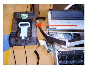
NOTE: When you reinstall the Carriage Assembly, take care not to damage the PRS Slider.
