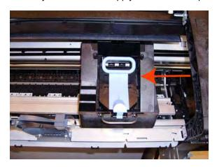
**15.** Remove the top T-15 screw that secures lnk Supply Tubes guide to the printer.
