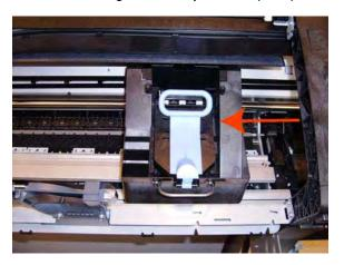
17. Remove the cover on each side of the Carriage PCA using a screwdriver unclip it.
