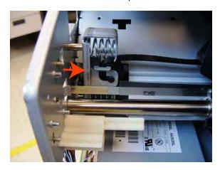
25. Remove the Belt Assembly from the Scan-Axis Motor drive wheel.
