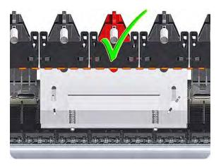
13. Fully tighten the two T-15 attachment screws that secure the Pinchwheel Assembly to the printer.
