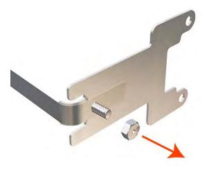
Remove the Encoder Strip Spring.
