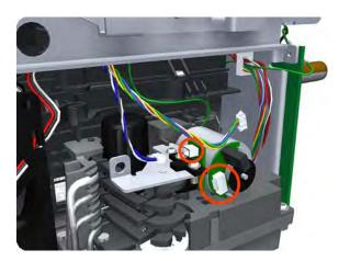
7. Unroute the cables disconnected in the previous two steps from the two cable clamps.
