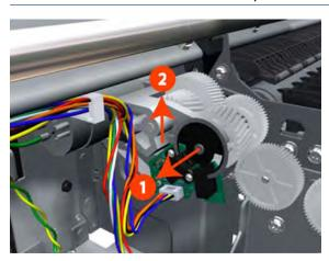
6. Disconnect the two Encoder Sensor connectors.
