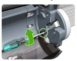
Detach the roll cover from the printer on the left-hand side. **5**.
