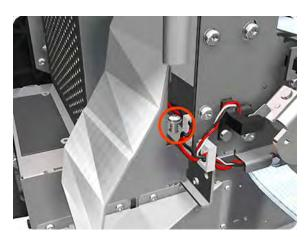
8. Remove two T-20 screws that secure the Electronics Module to the printer.
