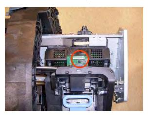
11. Remove the four T-15 screws that secure the Ink Supply Tubes to the Carriage Assembly.
