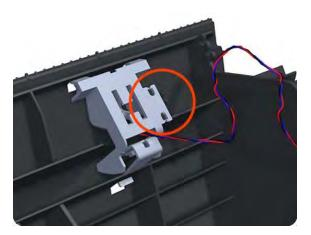
6. Press the clip to remove the Out Of Paper Sensor cover from the Clean Out Assembly.
