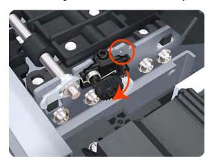
10. Tilt the Right Starwheel Lifter sufficiently to disengage the left attachment lug.
