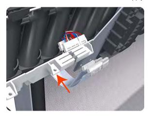
12. Carefully lift the Cartridge Tubes Connector out of the Left Ink Supply Station.
