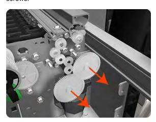
8. Remove three T-8 screws that secure the Starwheel Motor to the printer.
