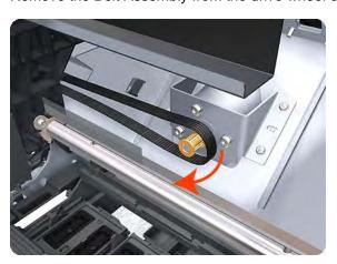
**9.** Remove three T-20 screws that secure the Scan-Axis Motor to the printer.
