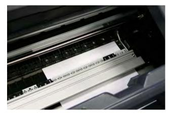
4. When you have loaded the paper, press **OK**. The printer starts the calibration process, and displays the results on the Front Panel if successful. Press **OK** to continue.
