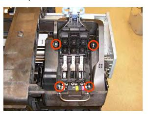
19. Carefully lift out the lnk Supply Tubes and close the carriage cover at the same time.
