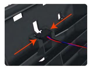
**10.** Lift the Out Of Paper Sensor out of the Clean Out Assembly.
