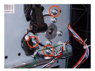
**13.** Carefully pull the Scan-Axis Motor out of the printer (10 mm) until you can rotate it approximately 30 degrees counterclockwise.
