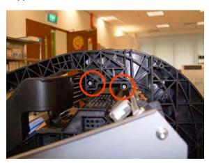
8. Carefully slide the Ink Supply Tubes Support Rail to the left until the right end is clear of the right Top Cover Support.
