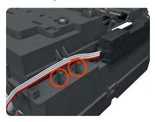
5. Remove the T-10 screw that secures the Drop Detector to the Service Station.
