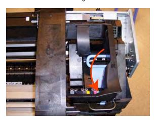
**11.** Carefully move the Ink Supply Tubes into the print path.
