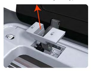
**5**. Remove the Damper Rotary from the Top Cover.
