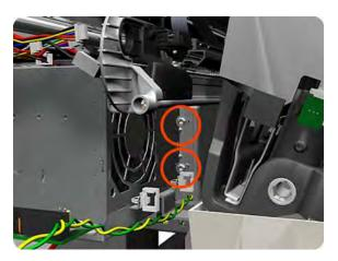
**6.** Remove one T-15 screw that secures the Electronics Module to the printer.
