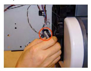
22. Push the Carriage Assembly into the print path.
