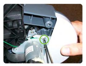
6. Remove two screws as shown.
