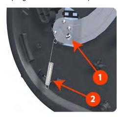
6. Remove three T-20 screws that secure the Media Lever.
