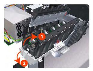
14. Carefully lift the Left Ink Supply Station completely out of the printer.
