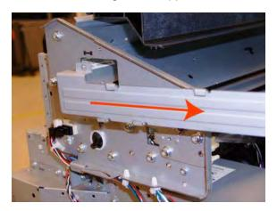
**31.** Remove the seven T-15 screws that secure the Scan Side Panel to the printer.
