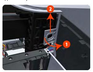
**10.** Remove the front T-15 screw that secures the front left side of the Top Cover to the printer.
