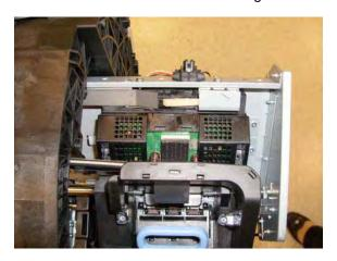
11. Disconnect the ribbon cable of the Trailing Cables from the Carriage PCA.
