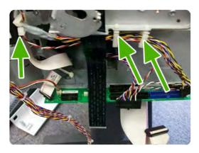
4. Remove ferrite from the FP cable without cutting the cable tie.
