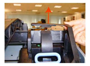
11. Straighten the ribbon cable of the Trailing Cables and remove the mylar.
