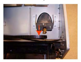
**26.** Remove the two T-10 screws that secure the Media Lever attachment plate.
