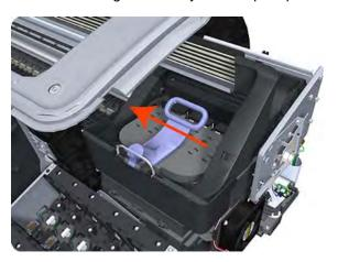
6. Remove one T-10 screw that secures the Drop Detector to the Service Station.
