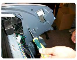
5. Unplug the Upper Left Roll Support, taking care not to damage the cables. Detach all cables from the Roll Support.
