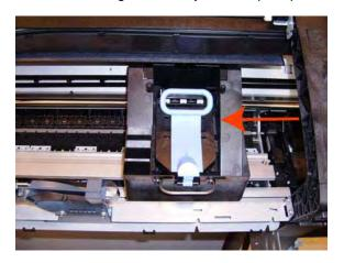
23. Loosen the T-15 screw Belt Tensioner to the printer to remove the tension from the belt.
