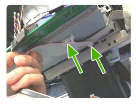
10. Unclip more cables from the cable ties.
