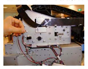
29. Unscrew the Trailing Cable support (two screws).
