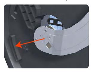
Remove the Media Lever from the printer.
