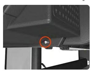
7. Remove one T-15 screw that secures the Right Cover to the printer (at the rear of the printer).
