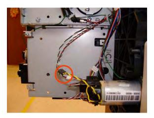
4. Unsnap the clamp from the bottom of the metal sideplate.
