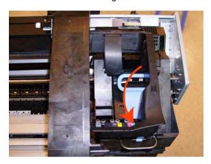
**14.** Carefully move the lnk Supply Tubes into the print path.
