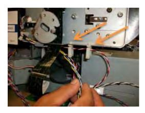
**8.** Remove the tape from the cable branch.
