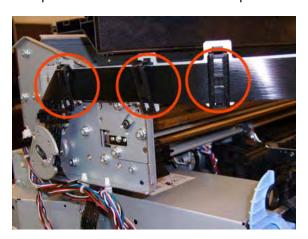
**18.** Pass the Trailing Cable through the slot.
