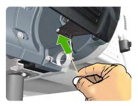
15. Free one end of the left metal link of the left Bi-stable Spring (if necessary, play slightly with the Lower Roll Cover).
