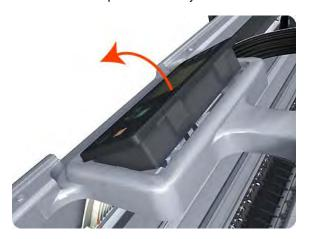
5. Disconnect the interface cable from the Front Panel.
