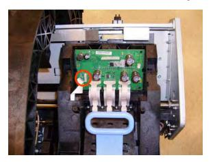
**14.** Remove four T-8 screws that secure the Carriage Assembly Cover hinge.
