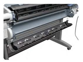
**10.** Hold the roll cover with one hand while unscrewing the bi-stable spring from the printer.
