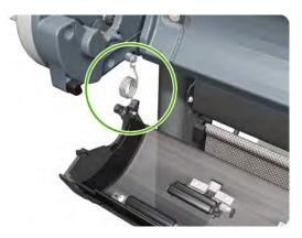
Detach the roll cover from the printer on the right-hand side.
