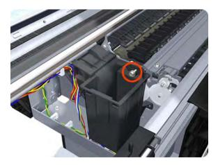
$\ensuremath{\textbf{4.}}$  Remove one T-8 screw that secures the Left Spittoon to the printer.
