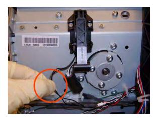
4. Disconnect the Pen to Paper Space (PPS) Solenoid connector from the L1 Data Harness.
