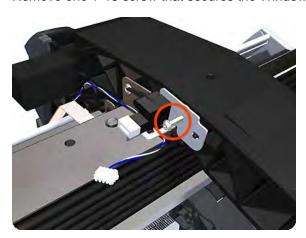
**9.** Remove the Window Position Sensor from the printer.
