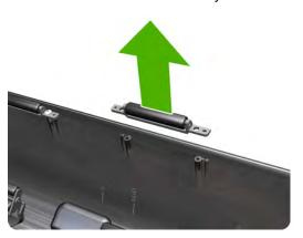
4. Locate the new freewheel assembly and screws.
