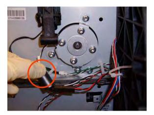
11. Disconnect the Scan-Axis Motor supply connector from the L1 Harness.
