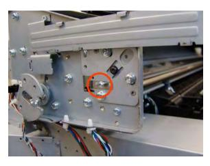
5. Grip the Encoder Strip and move it towards the left to take off the tension until you have completed the next step.
