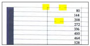
Below, the stepped lines highlighted in yellow are misdirected. When the line is misdirected, this means the nozzle is malfunctioning or out of position.
