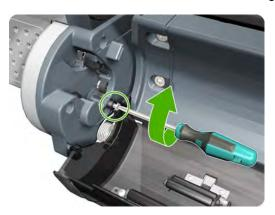
Screw the Lower Roll Cover to the Lower Left Roll Support. 8.
