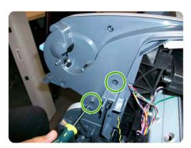
5. Unplug the Upper Right Roll Support, taking care not to damage the cables. Detach all cables from the Roll Support.
