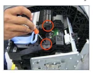
**18.** Disconnect the Line Sensor electrical connection from the Carriage PCA.
