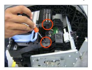
13. Disconnect all cables from the Carriage Assembly PCB.
