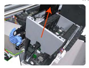
5. Remove two T-10 screws that secure the Right Side Plate of the Left Ink Supply Station.
