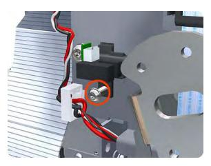
**6.** Rotate the Media Lever Position Sensor vertically to disengage the attachment lug from the Scan Side Panel.
