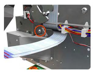
7. Remove one T-20 screw that secures the Electronics Module to the printer.
