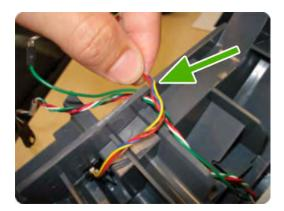
3. Push down the clip that holds the Siva sensor (you can use a screwdriver).
