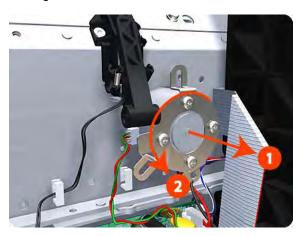
14. Remove the Scan-Axis Motor from the printer.
