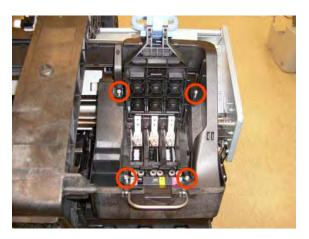
13. Carefully lift out the Ink Supply Tubes and close the carriage cover at the same time.
