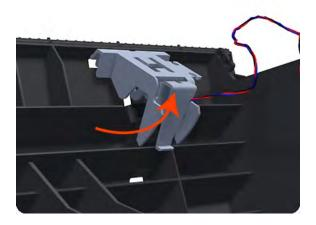
8. Remove the Out Of Paper Sensor cover from the Clean Out Assembly.
