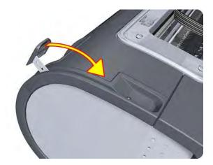
7. Make sure the Pinchwheel Alignment Tool is in the collapsed position.
