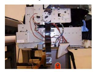
11. Unclip and remove the cable clamp of the Trailing Cables.
