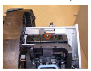
9. Remove the small cover of the Carriage PCA.
