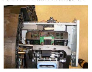
17. Disconnect the ribbon cable of the Trailing Cable from the Carriage PCA.
