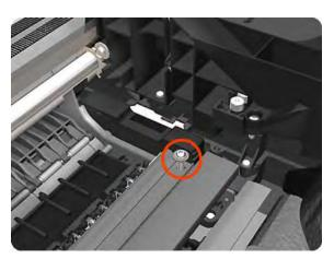
5. Carefully lift the Starwheel Assembly out of the printer.
