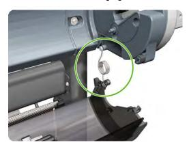
Both ends of the roll cover are now connected to the printer only by the bi-stable springs. 9.
