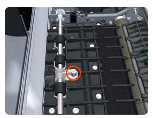
4. Lift attachment clamp vertically to release it from the Platen.
