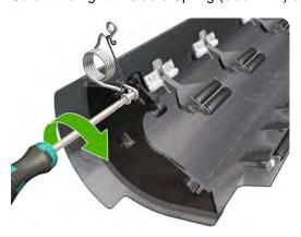
Screw the left Bi-stable Spring (gold link) onto the left side of the Lower Roll Cover.
