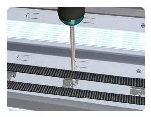
8. Remove two T-10 screws that secure the Pinchwheel Assembly to the printer.
