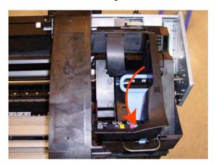
**21.** Loosen the T-10 uncapping screw sufficiently so you can manually move the Carriage Assembly in step 26.
