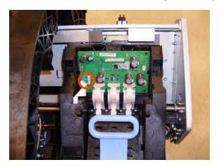
**14.** Press the locking clip to release the Carriage Assembly PCB from the carriage.
