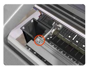
4. Remove another T-10 screw that secures the Starwheel Assembly to the printer.
