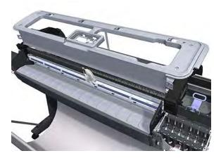
**13.** Unroute the Front Panel ribbon cable from the two cable clamps on the bottom surface of the Top Cover.
