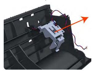
9. Squeeze the Out Of Paper Sensor attachment clips to remove it from the Clean Out Assembly.
