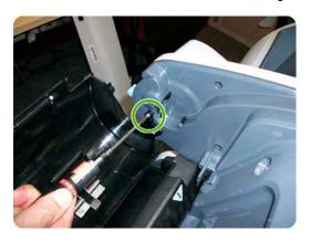
4. Remove the Roll Cover hinge from the Roll Left Support Pin.
