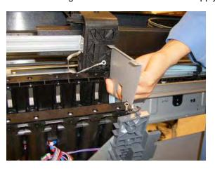
**24.** Carefully lift the Ink Supply Tubes out of the printer.
