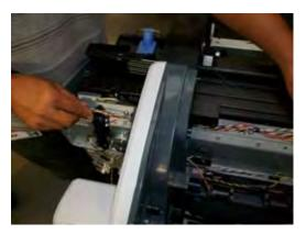
21. Back on the left side, detach the FP harness cable to leave space to detach the lower cable branch.
