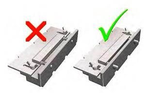
8. Fit the end of the Pinchwheel Alignment Tool to the Pinchwheel Assembly you need to align.
