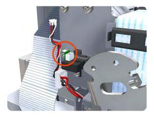
5. Remove one T-10 screw that secures the Media Lever Position Sensor to the Scan Side Panel.
