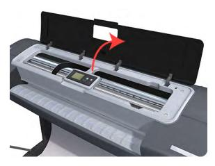
3. Remove the two T-15 screws that secure the left Window hinge locking plate to the Top Cover.
