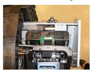
9. Disconnect the ribbon Trailing Cable from the Carriage PCA.
