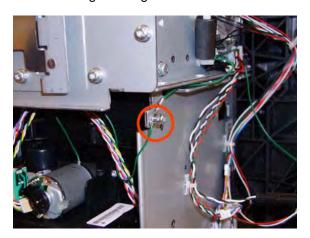
6. Disconnect connector from the Primer Motor and Primer Sensor.
