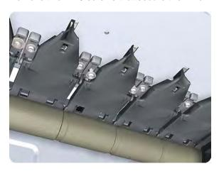
Remove the Pinchwheel Assembly from the printer.
