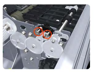
8. Rotate the Left Starwheel Lifter sufficiently to disengage the right attachment lug.
