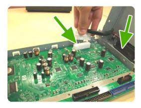
5. The PSU module has now been removed from the printer.
