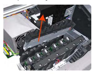
**13.** Carefully lift the Left Ink Supply Station enough so that you can rotate it counterclockwise to release the front attachment from the printer.
