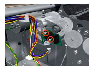
8. Remove the Encoder Sensor PCA from the printer.
