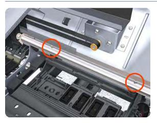
11. Unclip the clip to release the Service Station from the printer.
