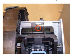
8. Remove the small cover of the Carriage PCA.
