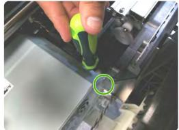
9. Unclip the ISS cable from the cable ties.
