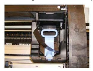
**13.** Slide the Trailing Cables out of the cable and tube holder.
