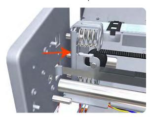
8. Remove the Belt Assembly from the drive wheel of the Scan-Axis Motor.
