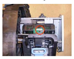
8. Remove the four T-15 screws that secure the Ink Supply Tubes to the Carriage Assembly.
