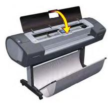
6. On the front panel, select the Ink icon, and then select Replace Printheads. The Carriage Assembly moves to the left and stops in the correct position to remove the printheads.
