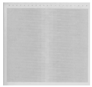
The following plot shows a bad media advance, there is a straight white line positioned close to the -6 column, instead of the 0 column for the majority of the points.
