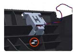
7. Rotate the Out Of Paper Sensor cover approximately 45 degrees.
