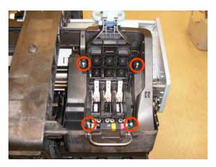
**12.** Carefully lift out the lnk Supply Tubes and close the carriage cover at the same time.
