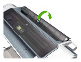
2. Remove the spindle.
