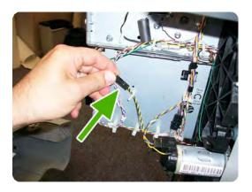
5. Remove the screw of the grounding cable.
