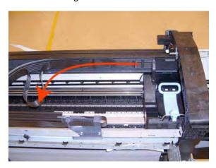
14. Disconnect the ribbon cable of the Trailing Cables from the Electronics Module.
