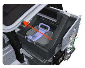
6. Loosen the T-20 screw Belt Tensioner to the printer to remove the tension from the belt.
