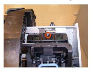
**16.** Remove the small cover of the Carriage PCA.
