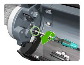
Remove the screw connecting the roll cover to the printer on the right.
