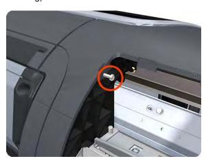
10. Remove one T-15 screw that secures the Left Cover (bottom rear).
