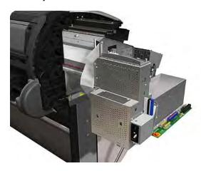
NOTE: When you install the Electronics Module, make sure it is correctly aligned with the mounting rail.
