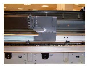
**18.** Use a flat-bladed screwdriver to release all the lnk Supply Tubes clamps from the printer.
