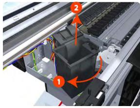
**5.** Rotate the Left Spittoon clockwise approximately 45 degrees and carefully lift it out of the printer.
