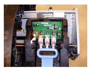
19. Carefully unroute the Line Sensor cable from the Carriage Assembly.
