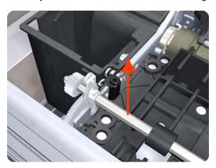
9. Slide the left Print Zone Overdrive to the left disengage the center coupling.
