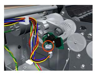
Remove two T-6 screws that secure the Encoder Sensor to the Media Advance Drive.
