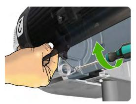
11. Screw the right pre-loaded Bi-stable Spring to the Lower Right Roll Support.
