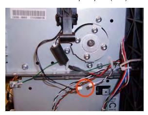
5. Remove two T-10 screws that secure the Pen to Paper Space (PPS) Solenoid to the printer.
