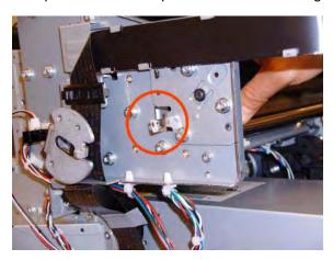
7. Loosen the T-10 uncapping screw sufficiently so you can manually move the Carriage Assembly in step 7.
