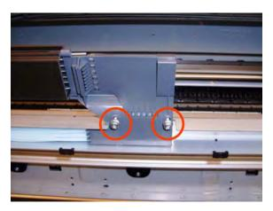
17. Carefully lift the Ink Supply Tubes guide enough until you can slide it forwards out of the printer.
