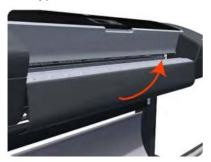
4. Unhook the Front Cover from the four attachments and remove it from the printer.
