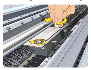
11. Allow the Pinchwheel Alignment Tool to expand. Make sure that the tool is fully expanded.
