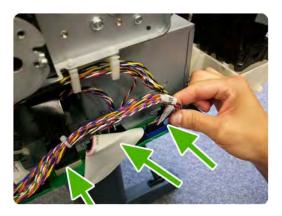
**3.** Unclip the cables from the cable ties.
