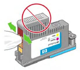
NOTE: Do not touch, wipe or attempt to clean the printhead nozzles. This can damage the printhead and reduce print quality.
