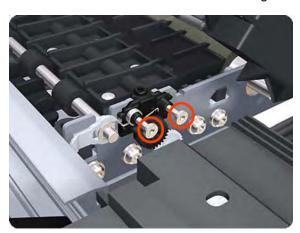
9. Rotate the Right Starwheel Lifter sufficiently to disengage the right attachment lug.
