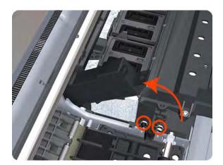
8. Remove two T-8 screws that secure the Right Starwheel Lifter to the printer.
