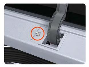
7. Remove the remaining three Window hinge locking plates from the Top Cover.
