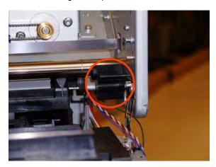
6. Remove the T-15 screw that secures the left bumper.
