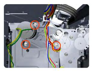
**8.** Grip the motor housing of the Media Advance Drive and gently pull it towards you sufficiently to allow you disengage the Media Advance Drive from the printer.
