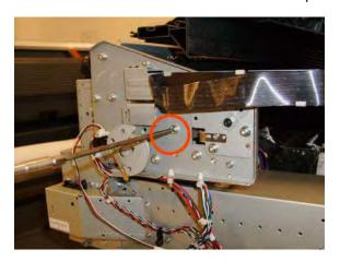
**24.** Leave the Belt Tensioner in place with all the tension removed.
