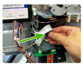
5. Unclip the cables from the cable ties.
