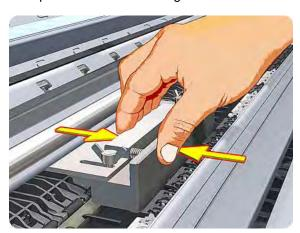
15. Remove the Pinchwheel Alignment Tool from the printer.
