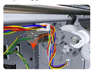
9. Carefully lift the Media Advance Drive out of the printer.
