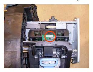
12. Remove the four T-15 screws that secure the Ink Supply Tubes to the Carriage Assembly.
