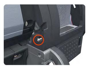
12. Remove one T-15 screw that secures the Left Cover (bottom front, accessible under Front Cover).
