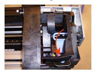
**15.** Loosen the T-10 uncapping screw sufficiently so you can move the Carriage Assembly manually.
