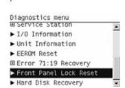
The Front Panel prompts you to unlock front panel access. Press OK to unlock access or Cancel to exit.
