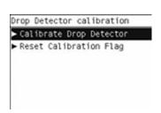
3. When the following message appears on the front panel, you must select whether you would like to continue with the calibration by pressing the **OK** key. Press **Cancel** to exit the calibration.
